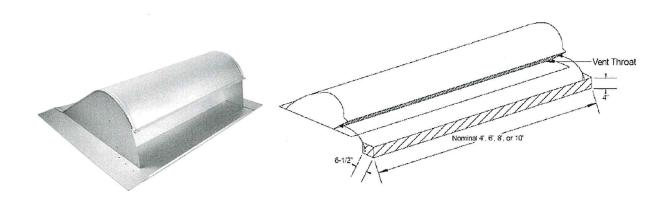
TAMCO Round Top Off-Ridge Vent with Baffle for Tile Minimum 26 ga. ASTM A792 AZ50 (non-HVHZ only) or ASTM A653 G90 galvanized steel off-ridge static roof ventilator with intake baffle for use with low-profile tile roof systems. Vent dimensions are 24" wide x 4-1/4" high and is available in nominal lengths of 4-ft, 6-ft, 8-ft and 10-ft. Material shall conform with FBC Section 1507.4.3 (non-HVHZ) and 1517.6 (HVHZ).
