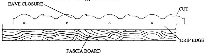
2. Closure overlaps approximately 1". Measure to next pattern then secure. Measurement same distance as between patterns on solid piece.
