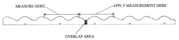
3. Tile has well defined recess in which closure is designed too lay.
