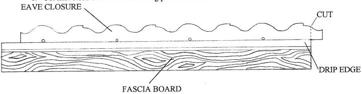
2. Closure overlaps approximately 1". Measure to next pattern then secure. Measurement same distance as between patterns on solid piece.
