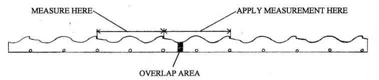
3. Tile rests on riser behind second ridge. Not designed to fit groove between first and second ridges.
