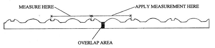
3. Tile sets on closure between the two ridges on tile bottom. Slide tile back until stopped by front ridge.
