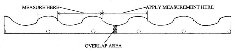
3. Tile has well defined groove in which closure is designed too lay.
