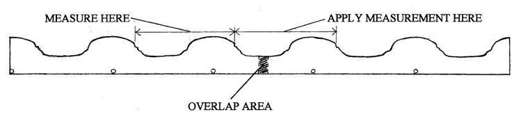
3. Tile has well defined groove in which closure is designed too lay.
