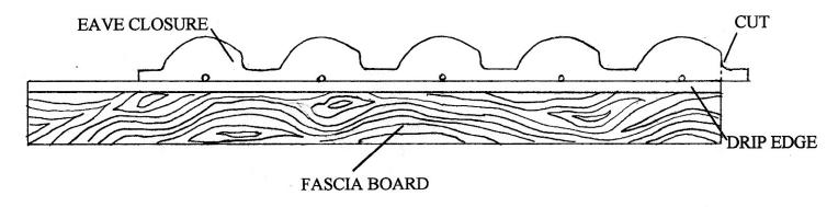
2. Closure overlaps approximately 1". Measure to next pattern then secure. Measurement same distance as between patterns on solid piece.
