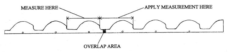
3. Tile overhang is measured to 1". There are no grooves or ridges that determine Tile positioning.
